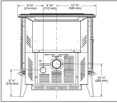
INSTALL VENT AT CLEARANCES SPECIFIED BY THE VENTING MANUFACTURER
